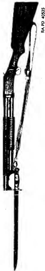
Figure 1—Gun with Bayonet, Hand Guard and Sling—Left Side View—Riot Type (Solid-Frame)— Winchester Shotgun M97
